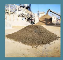
Concrete Treatment Machine was introduced aggregates. They can be reused as civil work materials or used in concrete production.
