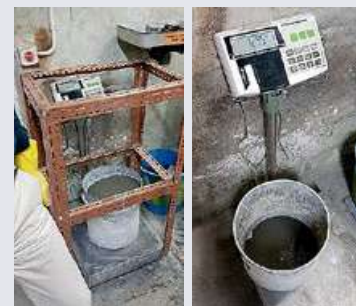
Segregation Resistance – Screen Stability Test 抗分離能力 – 篩分離測試
