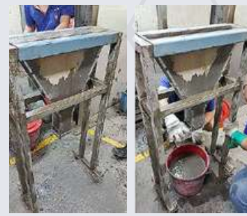
Viscosity – V-Funnel Test 黏度測試 – V型漏斗測試
