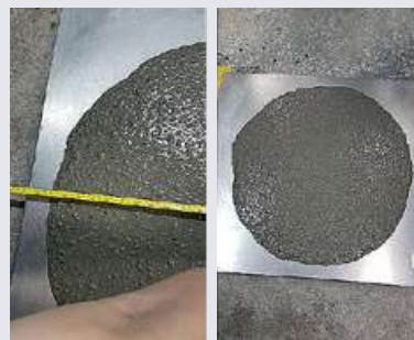
Flowability – Slump Flow Test 流動性 – 坍流度測試
