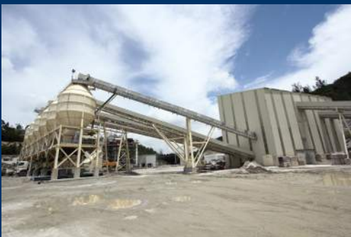
The fully enclosed production lines and materials delivery barge confined the transmission of pollutants to the surrounding environment and also isolated the noise generated from the machinery operations.
