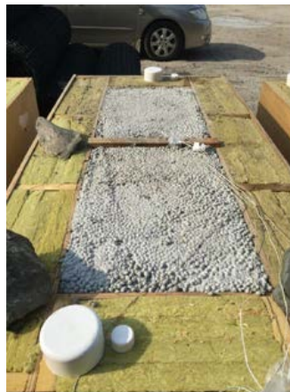
3. LECA-1 (Cement Content: 540 \text{ kg/m}^3 )
