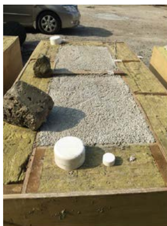
4. BST-3 (Cement Content: 600 \text{ kg/m}^3 )
