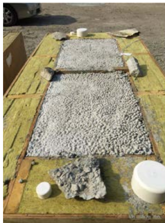
5. LECA-2 (Cement Content: 590 \text{ kg/m}^3 )
