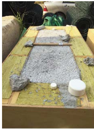
1. LECA 1A (Cement Content: 490 \text{ kg/m}^3 )
