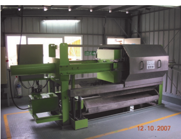
Filter press greatly reduced the water content in the solid waste
