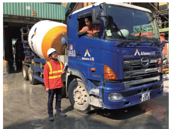
Inspection program to maintain truck cleanliness standard and to prevent muddy material and dust being carried to public roads
